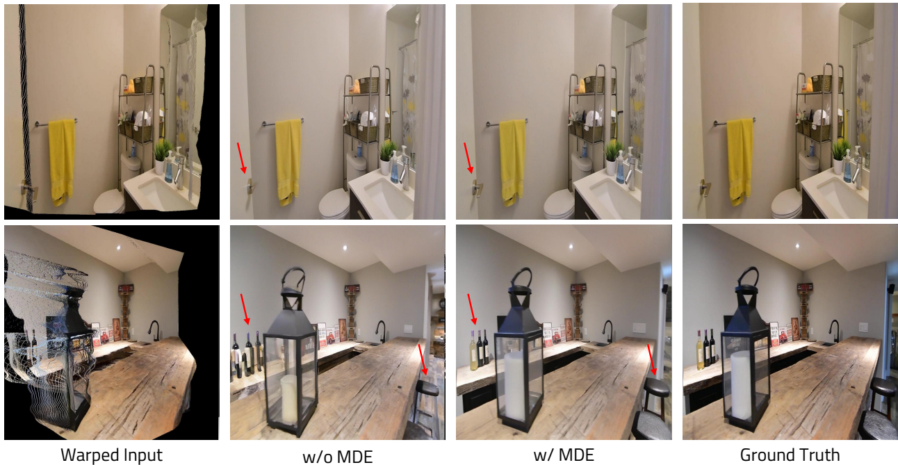
Figure 11. Qualitative comparison between two different conditional models. We train a warp-and-refine model without the monocular depth (MDE) condition. Without MDE supervision, the model struggles to correct local alignment issues ( e.g. , the door handle, wine bottles, and chairs), resulting in noticeable geometric distortions and texture artifacts. In contrast, incorporating MDE enables the model to leverage pixel-aligned depth cues and more faithfully reconstruct fine details, yielding sharper and more consistent multi-view results.
