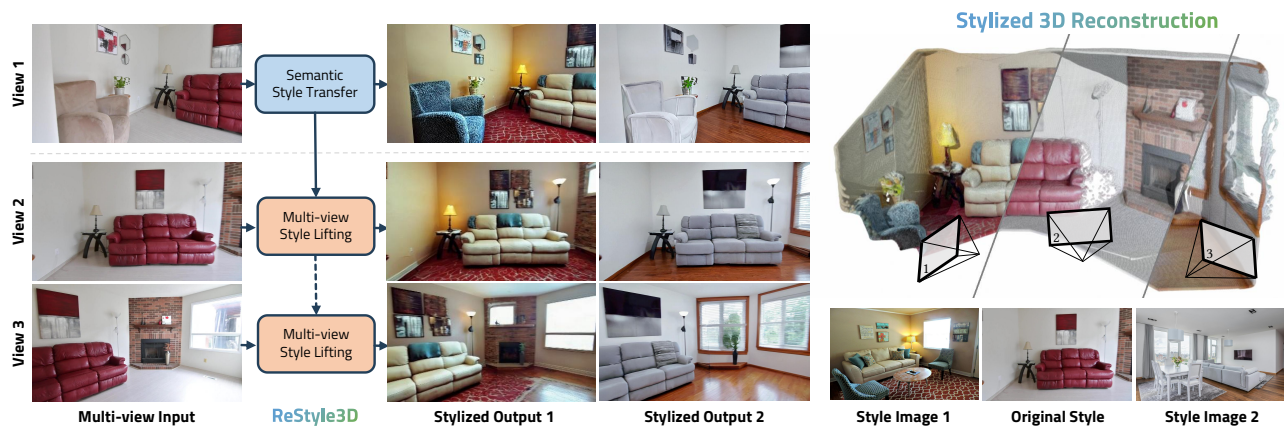
Figure 1. Given an interior design image (style image) and a 3D scene captured by video or multi-view images, ReStyle3D first transfers the appearance based on semantic correspondences to a single view, then lifts the stylization to multiple viewpoints using 3D-aware style lifting, achieving multi-view consistent appearance transfer with fine-grained details. Project page: restyle3d.github.io .
